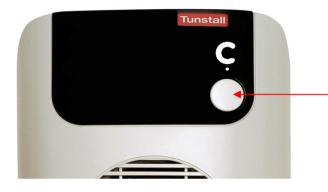
In addition to the red alarm button and privacy button, your speech module has a Cancel at Source button. If this button is not pressed after an alarm call is raised the speech module will continue to raise alarm calls.
