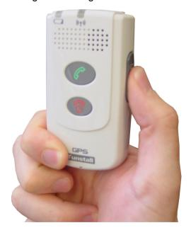
NOTE: The unit will try to find satellite signals for up to 1 minute.
