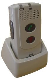
**NOTE:** If the MobilAlarm is properly seated in the charging base and the red indicator does not glow, then the unit may have been fully charged before being supplied to you.
