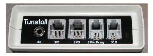
IP1 is used for the optional Extend Switch (41005/05)
