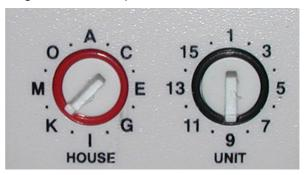
To set the address, simply insert a broad bladed screwdriver into the slot on the rotary switch, until the switch points to the desired address.
