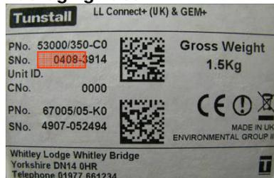
The week/year is identified using the first four digits of the home unit's serial number. This unit was manufactured in week 04 year 08.
